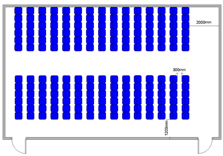
Layout and capacity based on the requirements of BS 9999: 2008 - Code of practice for fire safety in the design, management and use of buildings
